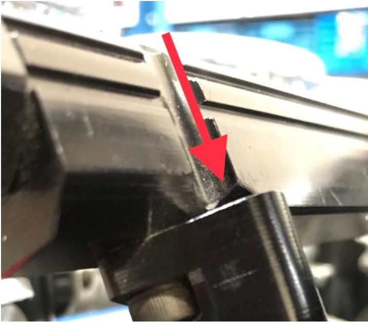
Figure 2: Correct 4mm socket head cap screw to remove
