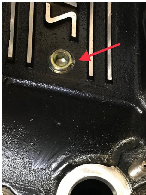
Figure 5: Set screw needs to be removed in order to connect downdraft to external vacuum canister
