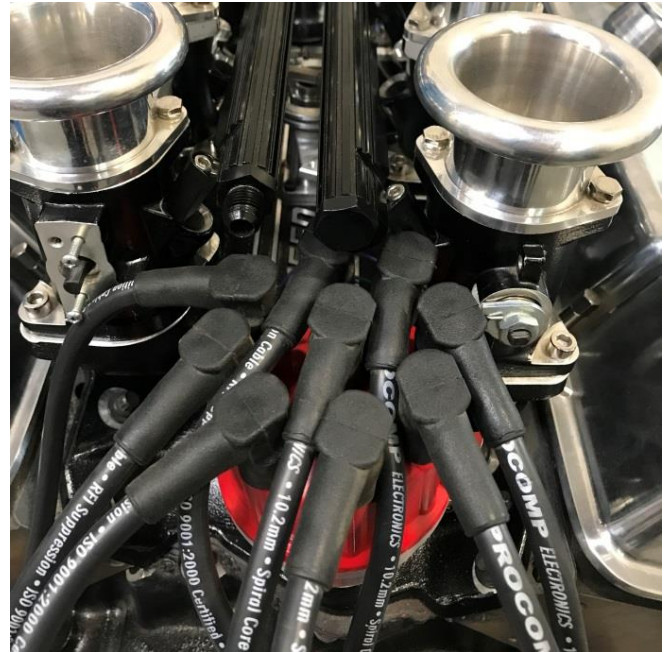
Figure 3: Fuel rail reinstalled after cap and wires are installed
