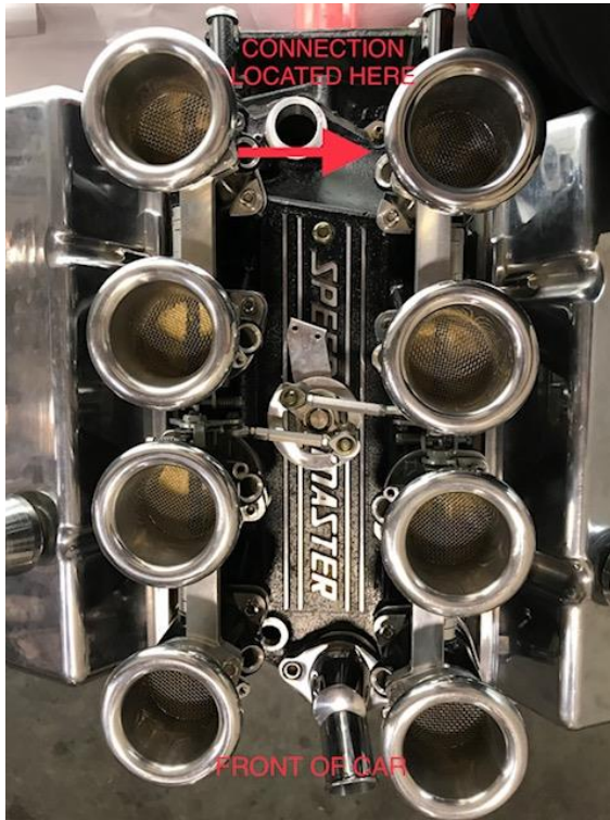
Figure 11: Top view of TPS location
